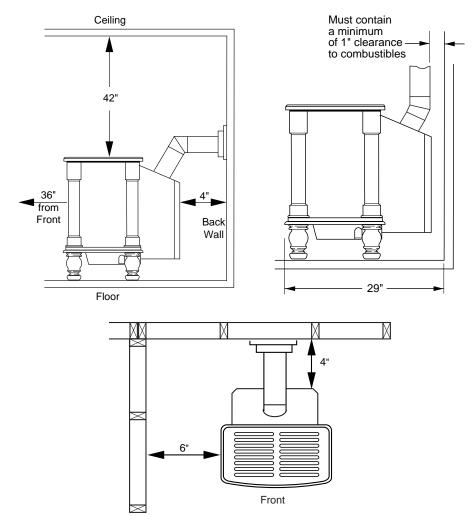
Figure 3 - Clearances for Standard Installation
